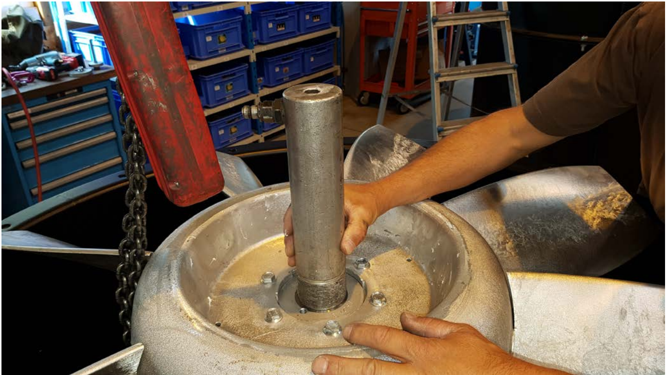
Step 8A: Put the two pulling rods with the pulley disk on top of the hydraulic cylinder
